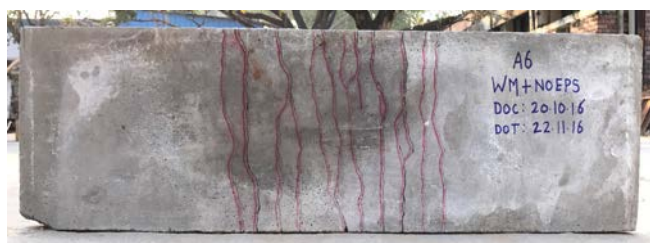
Fig. 5. Typical crack pattern for slab specimen S1
